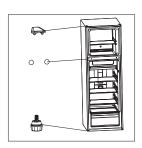
Step 10. Remove the hinge bushing and door stop of the R-door and F-door with screwdriver, and install them to the other side of the doors.
