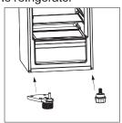
Step 11. Use a screwdriver to mount the middle hinge to the left side of the middle beam in front of the refrigerator
