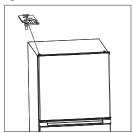
Step 2. Remove the top hinge with screwdriver
