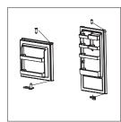
Step 12. Install the F-door onto the middle hinge.
