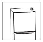
Step 4. Remove the middle hinge with screwdriver
