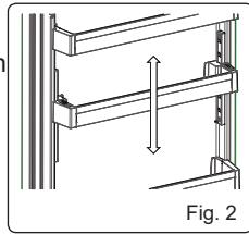
**Note:** Before moving door shelf is loaded, you must hold the shelf by supporting the bottom. Otherwise, door shelf could fall off the rails due to the weight. So damage may occur on the door shelf or rails.
