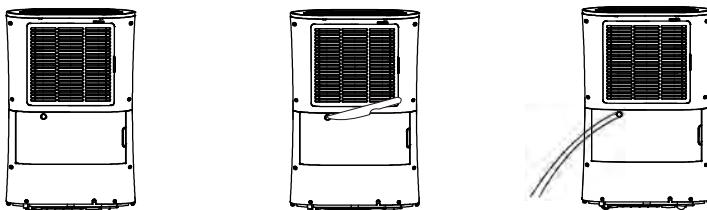
Make sure the connection between the pipe and the drain outlet is tight and does not leak. Then direct the pipe to a suitable drainage point. This unit uses gravity fall to dispose water hence the drain should be lower than the unit water outlet. Put the tank back. Be sure to run the water pipe downward and let the water to flow out smoothly. Do not kink or bend the pipe.
