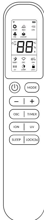
Press the timer button when the unit is in operation, to turn on/off the display of "clock +OFF" icon, it will flash 5", then press up/down button to adjust the 1-24h after which you want the unit to shut down. Press the timer button when the unit is in standby, to turn on/off the display of "clock+ON" icon, it will flash 5 seconds, then press up/down button to adjust the 1-24h and select the time to turn on.
